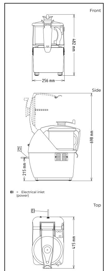
Electric Supply voltage: 200-240 V/1N ph/50/60 Hz **Electrical power max:** 1 kW 1 kW **Total Watts:** Capacity: Performance (up to): 2 kg/Cycle **Capacity:** 4.5 litres Key Information: External dimensions, Width: 256 mm External dimensions, 415 mm Depth: External dimensions, Height: 482 mm **Shipping weight:** 25 kg
